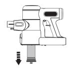
Ensure the appliance is switched off before cleaning, and remove the dirty pre-filter from the mesh filter-holder.
