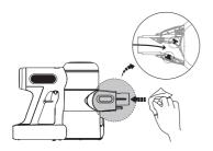
To avoid dust accumulation which can affect cleaning performance, wipe the suction mouth with a damp cloth.
