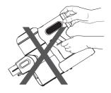
Do not place the appliance as above when removing or installing the HEPA filter, to prevent dust from entering the motor.
