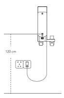
Determine the best wall location for mounting the dock. We recommend placing it 120cm from the lower screw hole to the floor (may need to be adjusted based on the actual situation).
