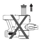
Do not turn the appliance upside down when removing or installing the filter to prevent dust from entering the motor.
