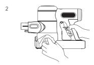
Clean with a damp cloth, taking care to prevent water entering the appliance main body and battery.
