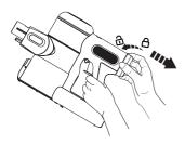
Turn the HEPA to the left and gently pull out for cleaning. Do not use the appliance without first installing the HEPA filter.
