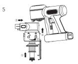
After cleaning, insert the clean pre-filter into the mesh filter properly and it clicks into place. Install the clean filter and dustbin back into the main body, then close the dustbin flap.
