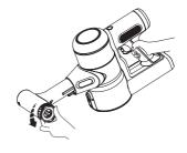
Run the appliance in MAX mode, and rotate the side cover to clean the dirty pre-filter.
